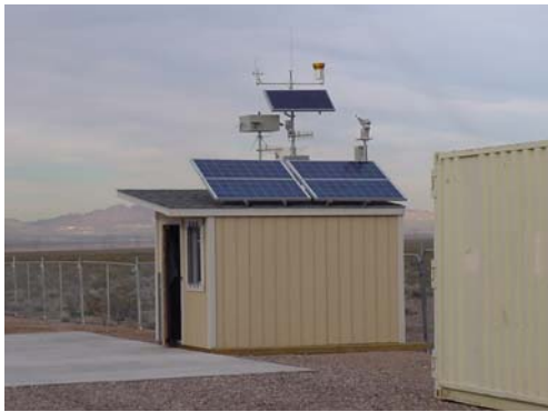
Figure 4. Instrumentation test shed located at the test site with camera box, weather station, Normal Incidence Pyrheliometer, and photovoltaic panels located on the roof.
